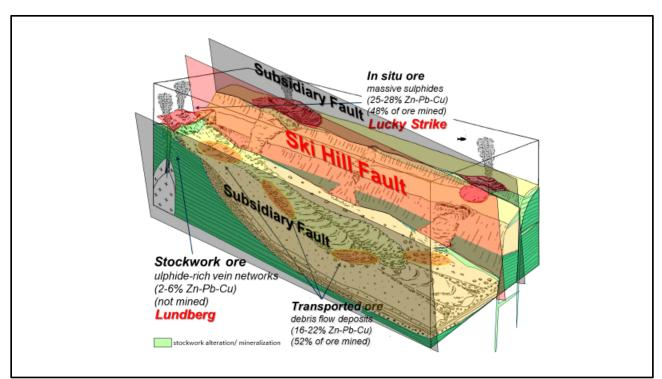
Figure 2 – Conceptualized model of the existing Buchans VMS mineralization that was mined along with the position of the current resources relative to a theorized VMS system (modified after Kirkham and Thurlow, 1987; and Thurlow, 2001).
