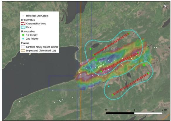
Figure 2: IP chargeability anomalies identifying the knowing massive-sulphide mineralization at long Lake and possible extensions of the known mineralization to the north and south. Historic gravity survey map shown with gravity highs in purple.
