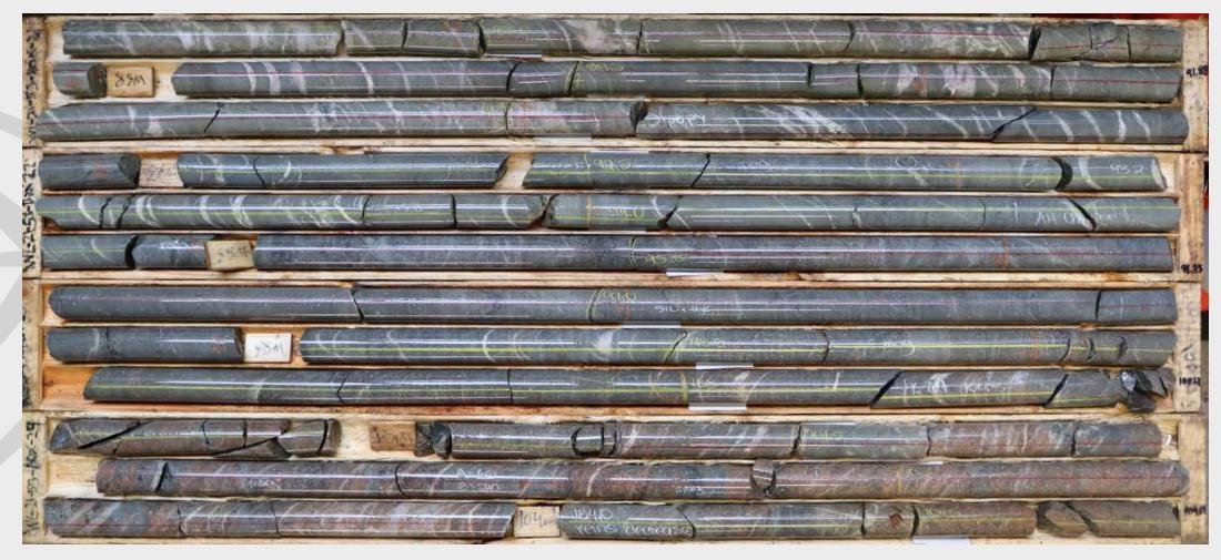
Multiple phases of alteration, veining, and sulphides in felsic volcanics from hole WL21-51
